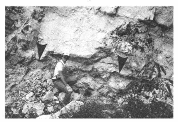
FIGURE 5 Stiff, fissured, plastic clay layer (8 cm thick).
