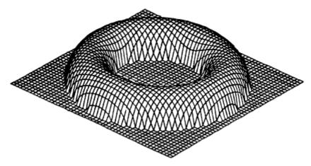
Figure 2.5 A perspective view of the surface of half-maximum magnetization density in the nucleus of vanadium-51. The diagram, computed from data obtained by the elastic scattering of electrons, reveals the circular orbit of the last valence nucleon in this nucleus. [From T. W. Donnelly and J. D. Walecka, *Nuclear Physics A201*, 81 (1973).]
