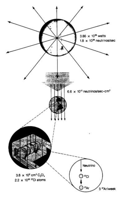
Figure 5.3 The solar-neutrino experiment being conducted in a South Dakota gold mine (see the text for details). Of every  $10^{22}$  neutrinos that pass through the 100,000 gallon tank of perchloroethylene, fewer than one interacts with a  $^{37}$ Cl nucleus. Each such interaction produces a  $^{37}$ Ar atom, which can be extracted and counted. The counting rate of about three neutrino-produced events per week is about one fourth the expected rate.
