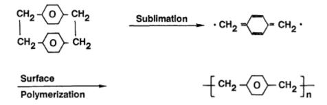
Adhesion is due to van der Waals interaction with the surface, and, while polyparylene films exhibit excellent chemical stability, poor adhesion continues to be a major technological problem and limitation. Surface modification techniques, which result in covalent interaction between the polymer film and the surface, might greatly improve adhesion and hence render polyparylene films more protective.
