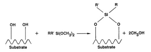
If R and R' are polymerizable groups, it is possible to form covalently bound polymeric coatings that have far superior adhesion than their physically adsorbed counterparts.
