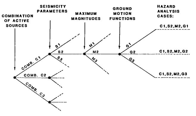
FIGURE 2.7 Example of logic tree format used to represent uncertainty in hazard analysis input. Each branch has an assigned weight and the sum of weights on branches attached to any node is unity (McGuire, 1986). Reprinted by permission from R. K. McGuire.
