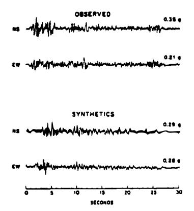
FIGURE 6.5 1940 Imperial Valley earthquake. Observed and simulated acceleration records at El Centro station (Munguia and Brune, 1984).
