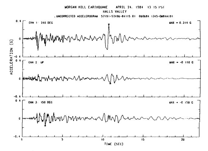
FIGURE 6.1 Processed data from the strong-motion records of the Morgan Hill Earthquake of 24 April 1984, Part I. ground-response records. (Office of Strong Motion Studies, 1986.)
