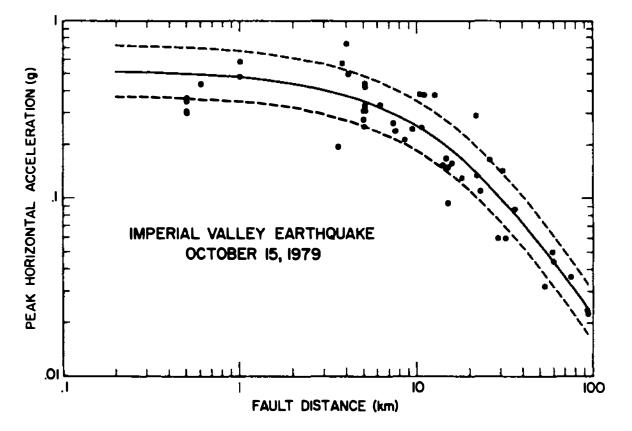
FIGURE 6.6 Observed and predicted mean horizontal peak accelerations for the 15 October 1979, Imperial Valley earthquake, plotted as a function of distance from the fault (Campbell, 1981).
