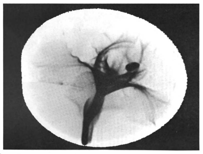
FIGURE 2-7. Real Time Radiography of an Iris.\* \*NOTE: The beetle just right of center.
