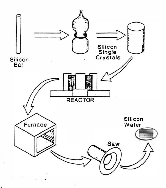
Figure 2-11. Doping Using Reactor Produced Neutron.
