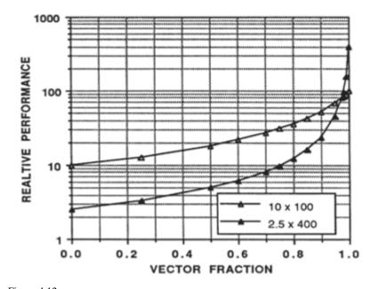
Figure 4.12 Balance in vector processor design. (Reprinted, by permission, from Worlton and Associates.)
