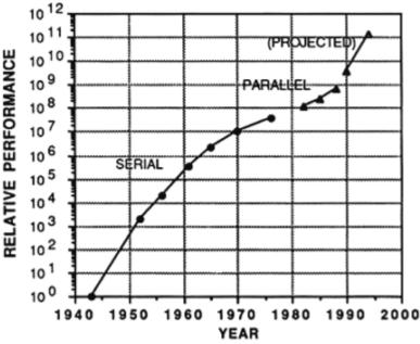
History and projection of execution rate at Los Alamos National Laboratory. Note: solid circle, serial; solid triangle, parallel; open triangle, projected. (Reprinted, by permission, from Worlton and Associates.)
