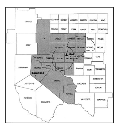
Figure 5 NOAA weather radio coverage—Midland/Odessa and Big Spring transmitters.
