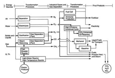
FIGURE 24.4 Functional diagram of an integrated energy system.
