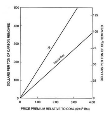
FIGURE 22.7 Cost of CO<sub>2</sub> reduction for fuel switching from coal to oil or gas.
