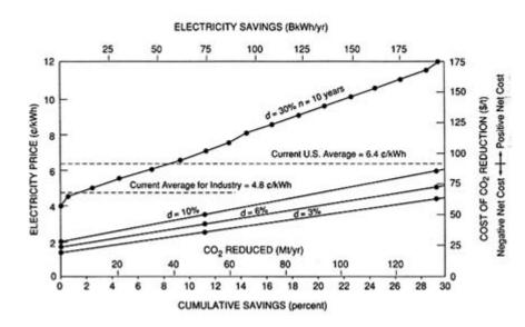
FIGURE D.5 Electricity conservation supply curve: Manufacturing (excluding energy management and cogeneration).
