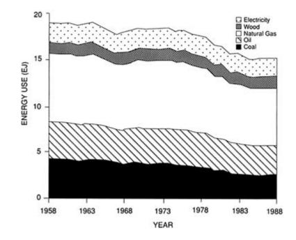
FIGURE 22.4 Impacts of structural changes on manufacturing energy use (activity and intensity fixed at 1973 levels).
