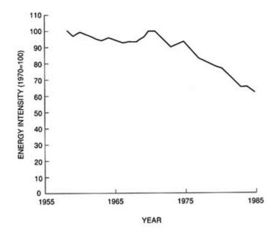
FIGURE 22.1 The aggregate energy intensity of U.S. manufacturing (relative to 1970). SOURCE: Ross (1989a).
