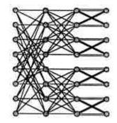
FIGURE 11.3: An 8-input 2-butterfly network. Reprinted, with permission, from Leighton and Maggs (1989). Copyright © 1989 by IEEE.
