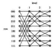
FIGURE 11.1: An 8-input butterfly network. Reprinted, with permission, from Arora et al. (1990). Copyright © 1990 by ACM Press.
