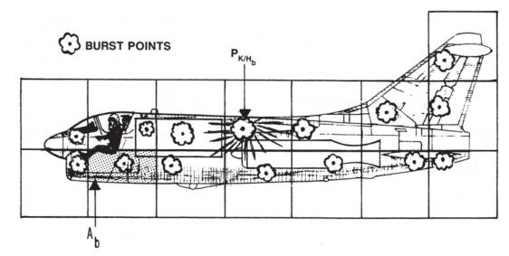
FIGURE 1-3 Grid cells and shotlines for the contact-fuzed high explosive weapon (Ball, 1985). Copyright © AIAA 1985—Used with permission.
