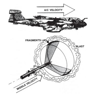
FIGURE 1-4 Aircraft vulnerability to the externally detonating HE warhead (Ball, 1985). Copyright © AIAA 1985—Used with permission.
