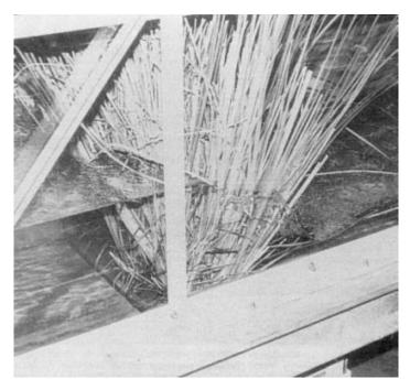
Oxford, Mississippi. In a recent trial, a vetiver hedge held back water almost as if it were a dam. This test was conducted in a flume (61 cm wide) and the water (flowing at 28 liters per second) was ponded to a depth of 30 cm behind the hedge. This result was all the more remarkable because the hedge was young and less than 15 cm thick. (Sedimentation Laboratory, Agricultural Research Service, U.S. Department of Agriculture)
