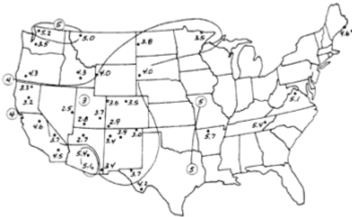
Figure 2-5 Average fine-particle absorption coefficient ( \text{Mm}^{-1} ) from the National Park Service network, 1983–1986. Fine elemental carbon concentrations in \mu\text{g}/\text{m}^3 can be estimated by dividing the fine-particle absorption coefficient (in \text{Mm}^{-1} ) by 10. Source: Eldred et al., 1987 (From Trijonis et al., 1990).
