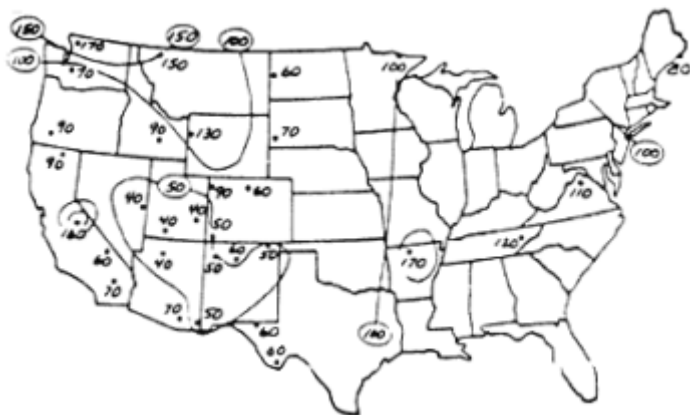
Figure 2-7 Average concentrations of fine-particle nonsulfate hydrogen mass ( \text{ng}/\text{m}^3 ) from the National Park Service network, 1983–1986. The nonsulfate hydrogen is calculated from the total hydrogen concentration by subtracting the hydrogen that is associated with sulfates. Source: Eldred et al., 1987 (From Trijonis et al., 1990).
