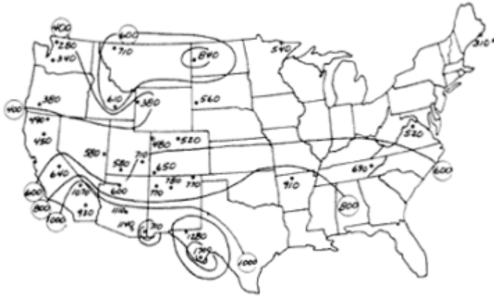
Figure 2-4 Average concentrations of fine-particle soil materials ( \text{ng}/\text{m}^3 ) from the National Park Service network, 1983–1986. Source: Eldred et al., 1987 (From Trijonis et al., 1990).
