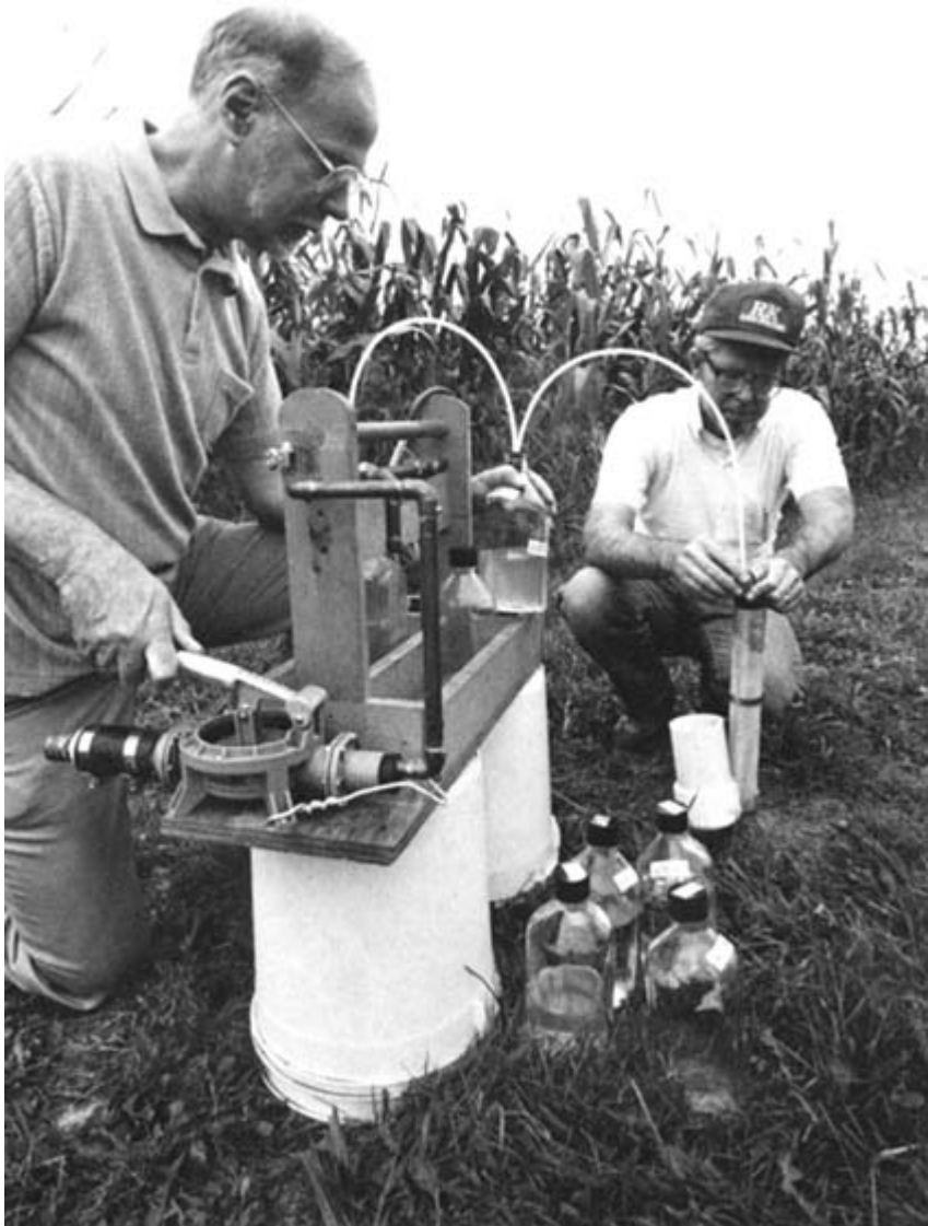
A chemist and a soil scientist with the Agricultural Research Service are studying the effect of different tillage systems on the movement of pesticides into groundwater. Here they take groundwater samples from a test site next to cropland at Beltsville, Maryland. Credit: Agricultural Research Service, USDA.
