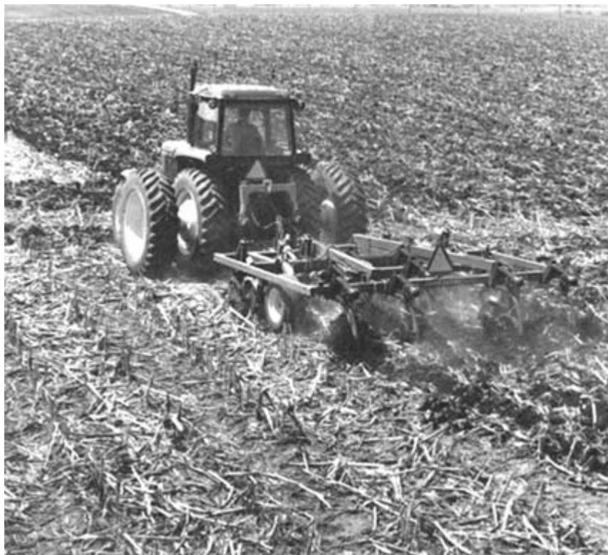
To prepare the soil for planting, this mulch tiller is designed to penetrate mulch cover. The mulch protects the soil from erosion and supplies organic matter to the soil. Credit: Deere & Company.
