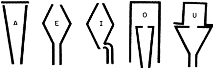
FIGURE 2 Kratzenstein's prize-winning implementation of resonators to simulate human vowel sounds (1779). The resonators were activated by vibrating reeds analogous to the vocal cords. The disparity with natural articulatory shapes points up the nonuniqueness between sound spectrum and resonator shape (i.e., job security for the ventriloquist).
