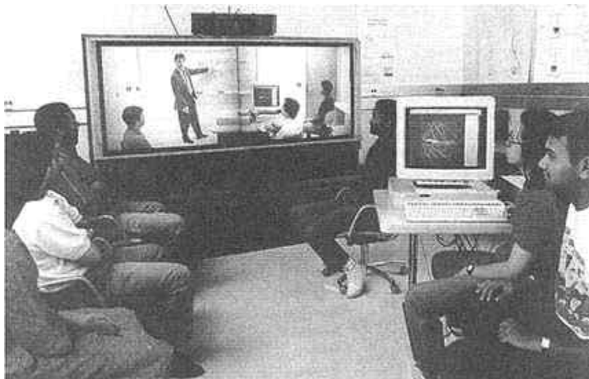
FIGURE 15b Large-screen video projection lends presence for group conferencing and instruction. Auto-directive microphone arrays permit hands-free sound pickup. System features are controlled by automatic recognition of spoken commands. Access to privileged data can be controlled by face and voice recognition for authorized individuals.
