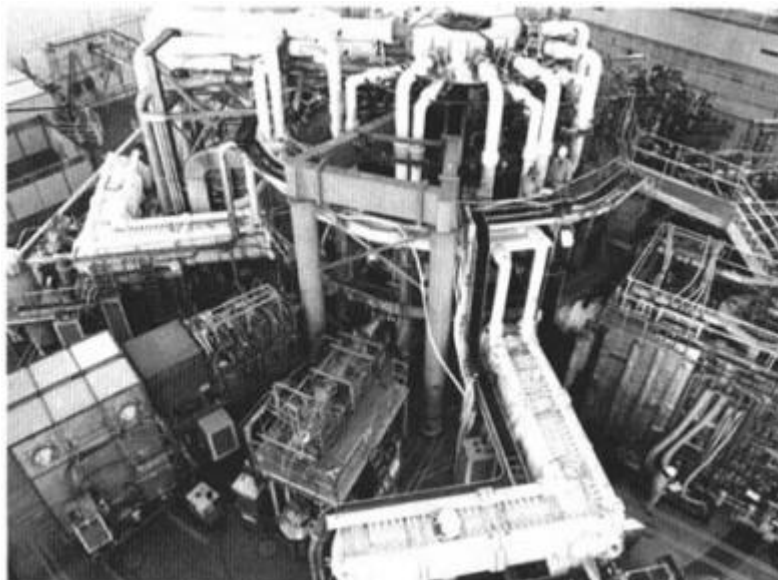
FIGURE 4.3 Photograph of the Tokamak Fusion Test Reactor (TFTR), located at the Princeton Plasma Physics Laboratory. The major radius of the donut-shaped plasma is 2.5 m. Typical plasma currents are 2.5 MA at toroidal magnetic fields of 52 kG. Powered by intense neutral beams and with a deuterium-tritium fuel mixture, TFTR has achieved record ion temperatures of 44 keV and fusion powers of 10.7 MW in second-long pulses. (Courtesy of Princeton Plasma Physics Laboratory.)
