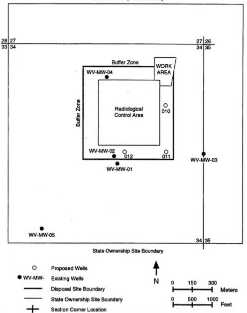
Figure 2.4 Relationship of various proposed Ward Valley site boundaries, and location of proposed and existing monitoring wells (after LA Figure 2420-4).
