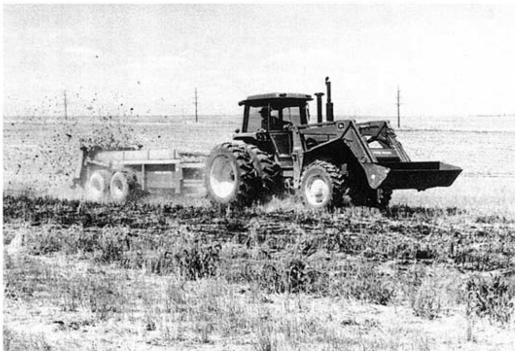
A tractor spreading sewage sludge on a stubble field before the growing season (photo courtesy of Robert Bastian, U.S. Environmental Protection Agency).
