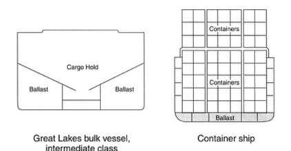
FIGURE 2-1 Typical ballast tank arrangements.
