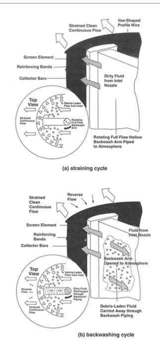
FIGURE 4-1 Operation of a self-cleaning strainer. Source: Adapted from Hayward Industrial Products, Inc. (1995).
