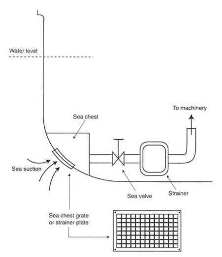
FIGURE 2-2 Typical ballast system.
