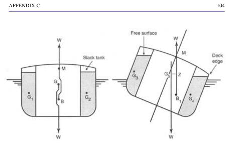
FIGURE C-3 Reduced GM with slack tanks (free surface effect).
