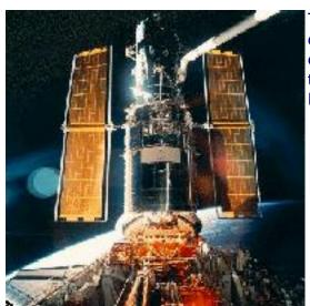
The Hubble Space Telescope orbit is always decaying due to atmospheric drag. Increased atmospheric densities in low-Earth orbit from solar-cycle-enhanced solar ultraviolet emissions and geomagnetic disturbances hasten the decay for this and other satellites (courtesy of Students for the Exploration and Development of Space).
