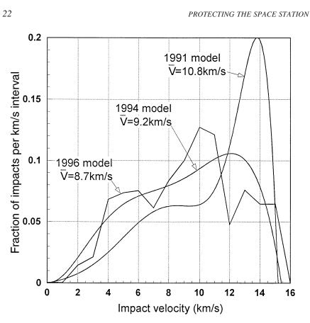
FIGURE 3-3 Comparison of model impact velocity predictions. Source: NASA.
