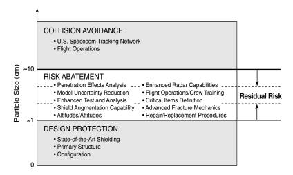
FIGURE 2-3 The ISS strategy for meteoroid/debris risk mitigation. Source: NASA.
