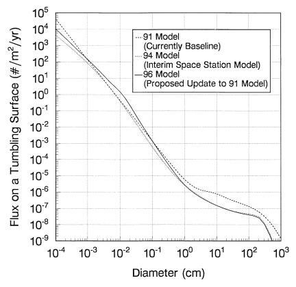
FIGURE 3-2 Comparison of model flux predictions. Source: NASA.
