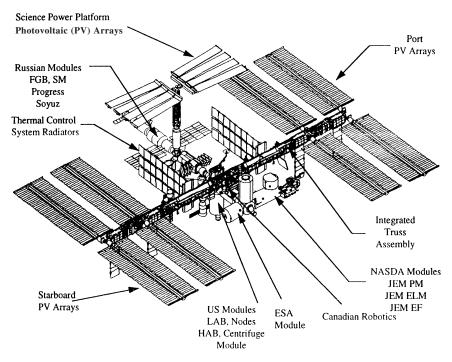
FIGURE 1-1 The International Space Station. Source: NASA.
