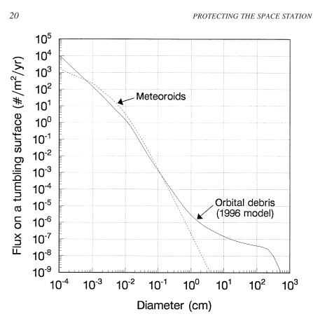
FIGURE 3-1 Comparison of meteoroid and debris flux in ISS orbit. Source: NASA.
