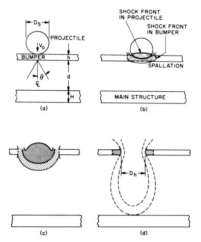
FIGURE 4-1 Projectile interacting with a spaced shield. Source: Riney.
