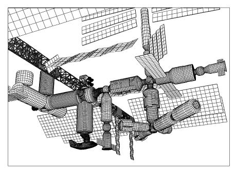
FIGURE 2-5 BUMPER finite element model of the ISS. Source: NASA.
