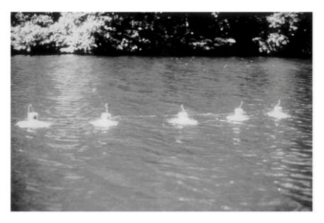
Gas sampling array for monitoring methane flux from lake and reservoir sediments through the water and into the atmosphere. There is growing evidence that lake and reservoir sediments are a major carbon sink worldwide. Source: U.S. Geological Survey.
