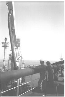
After the vessels are moored together, hoses are passed from the service vessel to the STBL and connected to the cargo oil piping.
