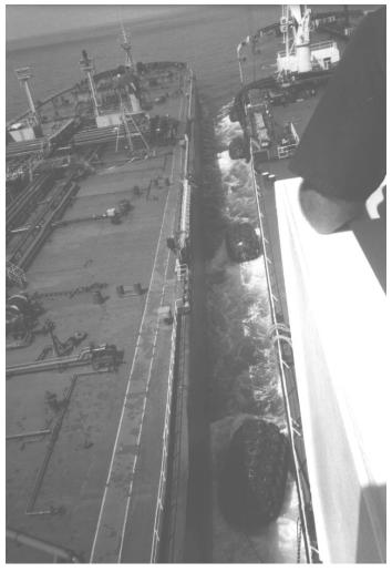
Fenders are deployed between the STBL and the service vessel.
