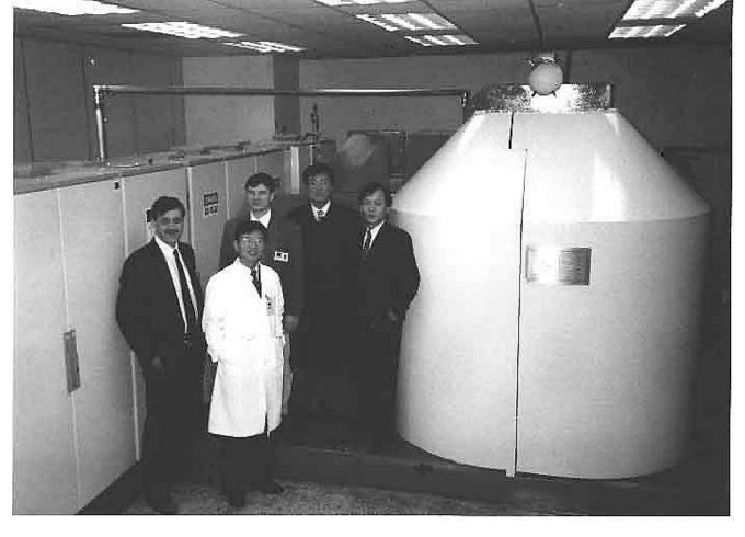
FIGURE 5-3 Photograph of the Ebco TR19 cyclotron accelerator. This machine is the same as the TR9D cyclotron accelerator proposed for the MDNR except that it generates 19 MeV protons rather than neutrons. Source: Tensor Technology, 1998a.
