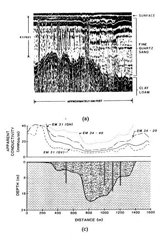
FIGURE 3.1 Examples of stratigraphic interpretations using subsurface geophysical surveys: (a) ground penetrating radar (from Benson et al., 1982); (b) delineating a bedrock channel by seismic reflection (from Benson, 1991); (c) relationship of EM
