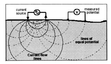
FIGURE 4.2 Schematic of a resistivity survey.
