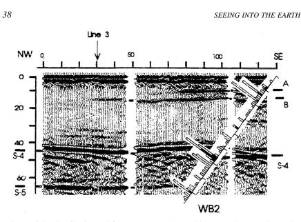
FIGURE 3.2 Semihorizontal fracture zones observed by ground penetrating radar along a profile measured on granitic outcrops at the Underground Research Laboratory, Manitoba, Canada, showing distribution of fractures along borehole WB2. Reflectors S-4 and S-5, seen at depths of 40 to 50 m and 65 m, respectively, are verified by increased fracture frequency observed in the slanted borehole. (From Holloway et al., 1992).
