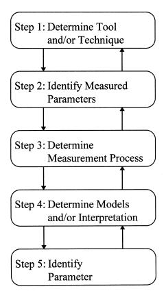
FIGURE 1.2 Steps in noninvasive parameter identification
