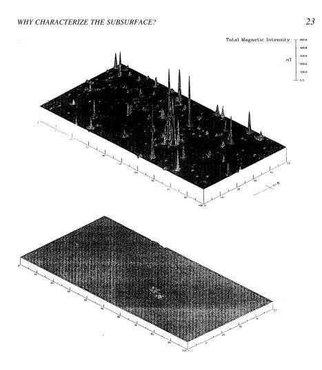
FIGURE 2.2 High-resolution magnetic survey for UXO detection
