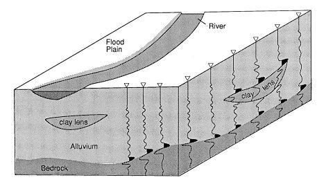
Simplified cartoon showing the "mapping" of bedrock and other fea-FIGURE 4.5 tures by seismic waves traced to individual geophone receivers.
