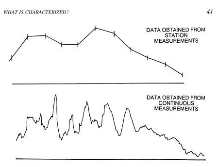
FIGURE 3.4 Comparison of station and continuous surface EM conductivity measurements made along the same transect. The electrical conductivity peaks are due to fractures in gypsum bedrock. (From Benson et al., 1982.)
