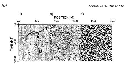
FIGURE 5.3 Visibility of GPR reflections decreases as the signal-to-noise (S/N) ratio increases; (a) is for S/N of 15.0, (b) for S/N of 7.5, and (c) for S/N of 1.5. T is the reflection from the top of a buried tank, B from the bottom of the tank, and F from a fluid (air/gasoline) interface inside the tank. Figure is from Zeng and McMechan (1997).
