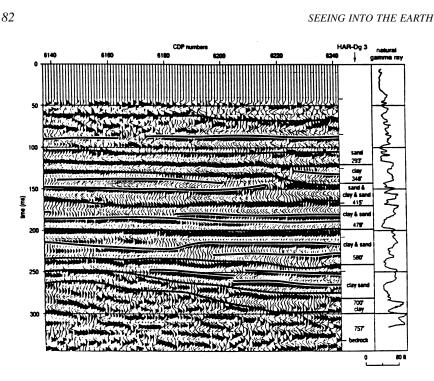
FIGURE 4.9 Seismic reflection profiling for geological variability.
