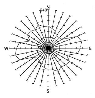
FIGURE 3.3 Resistivity measurements made in 16 different directions define a resistivity ellipse whose major axis is aligned with the fracture orientation. This example, from an open-pit quarry in southern Indiana, demonstrates that the dominant fracture direction is east-west. (From Cohn and Rudman, 1995.)
