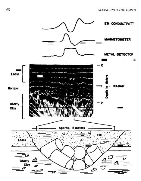
FIGURE 3.6 Buried metallic drums with representative magnetic and EM signatures; GPR signals show disturbed ground and surrounding stratigraphy. (After Benson and Glaccum, 1980.)
