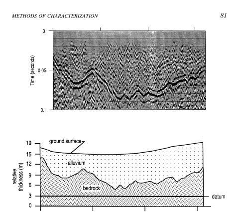
FIGURE 4.8 Seismic reflection cross section and interpreted cross section. The purpose of the characterization was to determine the placement of a monitoring well, which was designed to be placed at the deepest bedrock-alluvium contact. From D. Steeples.
