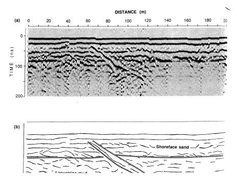
FIGURE 4.3 GPR profile along the escarpment of the Slave River Valley, Fort Smith, North West Territories, Canada. Early Holocene wave-influenced deltaic deposits with possible postdepositional slumping. (From Jol and Smith, 1992.)
