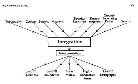
FIGURE 5.1 Schematic diagram of the concept of integrating geologic information and data from diverse geophysical methods for determining properties of a landfill. (After Roberts et al., 1989.)
