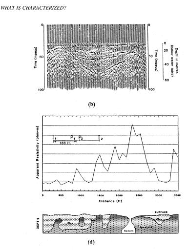
conductivity data and a sand and gravel channel (from Hoekstra and Hoekstra, 1991); and (d) electrical resistivity profile of karst terrain (from Hoekstra and Hoekstra, 1991). (Figure adapted from Cohen and Mercer, 1993).
