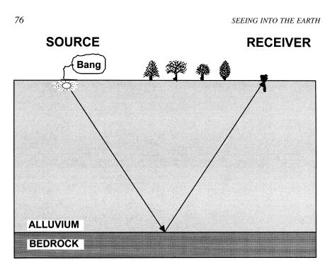
FIGURE 4.6 Simple reflection from bedrock. Either a seismic wave-velocity contrast or a mass density contrast is required for seismic waves to be reflected from the geological interface.
