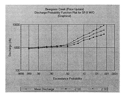
FIGURE 5.4 The flood-frequency curve and its uncertainty at damage reach SF-9 on the South Fork of Beargrass Creek.
