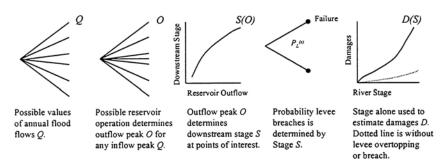
FIGURE 4.1. Event tree describing the transformation of flood discharge into damage. Some of the steps in this process are deterministic; others are stochastic. SOURCE: NRC (1995).
