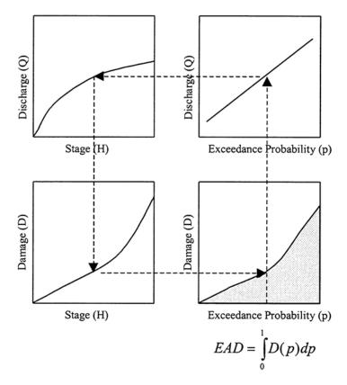
FIGURE 4.2 Basis of the Corps's computation of expected annual damage (EAD). The logic of this figure flows counterclockwise starting from the upper right panel and ending in the lower right panel. SOURCE: Adapted from Moser (1997).
