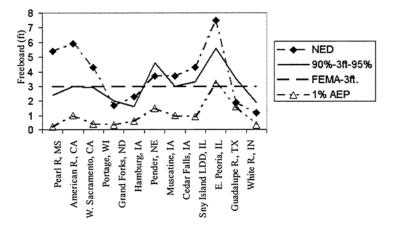
FIGURE 7.3 Comparison of freeboard requirements for the National Economic Development plan elevation and those arising from the levee certification criteria.
