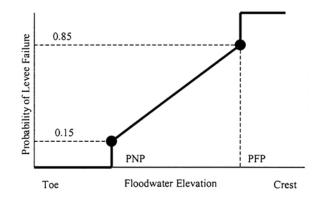
FIGURE 4.8 Two-point model of geotechnical levee reliability. PFP is probable failure point; PNP is the probable nonfailure point.
