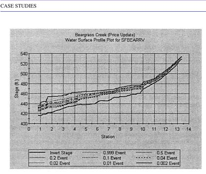
FIGURE 5.5 Water surface profiles for design floods in Beargrass Creek under existing conditions.
