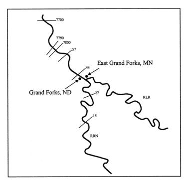
FIGURE 5.10 Schematic of the Red River of the North (RRN) and Red Lake River (RLR) at the East Grand Forks, Minnesota and Grand Forks, North Dakota study area. Numbers indicate USGS stream gages.
