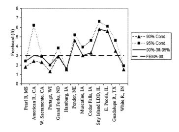
FIGURE 7.2 Current Levee Certification Criterion (90%-3ft-95%) and the FEMA Standard Three Feet.
