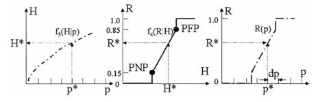
FIGURE 4.10 Computation of risk measures including geotechnical reliability.
