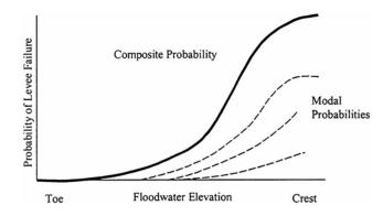
FIGURE 4.9 Continuous model of geotechnical levee reliability.
