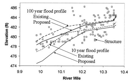
FIGURE 6.5 Comparison of water surface profiles for existing conditions and with a proposed flood damage reduction plan. This profile is from damage reach SF-9, Beargrass Creek.
