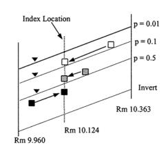
FIGURE 5.7 Assignment of structures to an index location.
