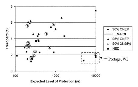
FIGURE 7.4 The expected level of protection provided by levee freeboard.
