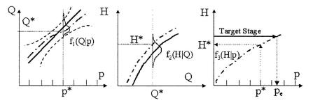
FIGURE 4.7 Computation of risk measures using a target stage.
