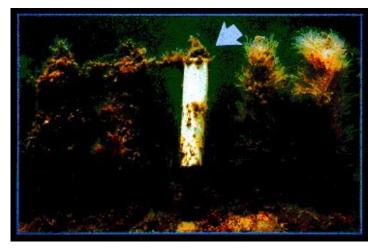
FIGURE 2. Photograph of a furanone-containing panel (center), with control panels, which had been exposed to the marine environment of Sydney Harbor for 5 months. Note the failure of marine biota in colonizing this material containing the natural blocking analog of the homoserine lactone signal that controls biofilm formation in many Gram-negative organisms. Reproduced with permission from Staffan Kjelleberg.
