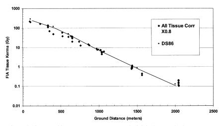
FIGURE 2-13 Nagasaki TL measurements (corrected). Original reported units—roentgens, tissue, air, quartz—converted to FIA tissue kerma (Cullings 2000).
