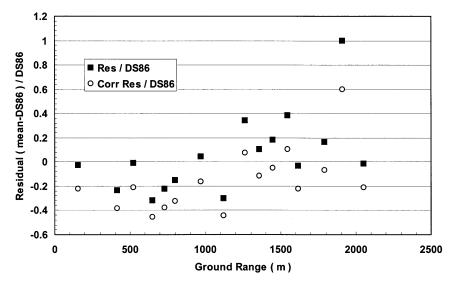
FIGURE 2-15 Hiroshima residuals (mean - DS86)/DS86; original measurement values and values corrected by 0.8.
