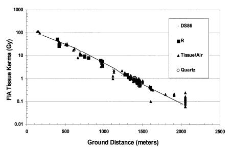
FIGURE 2-10 Hiroshima TL measurements. Original reported units—roentgens, tissue, air, quartz—converted to RA tissue kerma (Cullings 2000).
