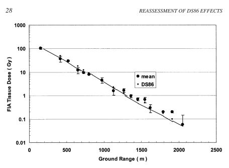
FIGURE 2-14 Hiroshima TL measurements averaged over 100-m intervals.
