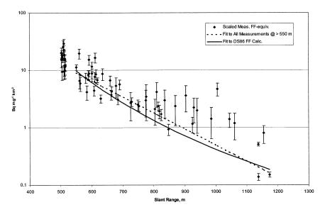
FIGURE 3-7 Nagasaki <sup>152</sup>Eu. The error bars are 1 SD.
