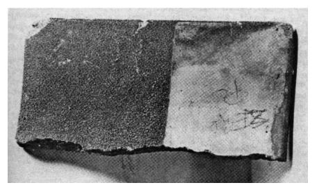
FIGURE 2-3 Blistered surface of roof tile; left portion of the tile was shielded by an overlapping one (0.37 mile from ground zero at Hiroshima) (Glasstone and Dolan 1977).
