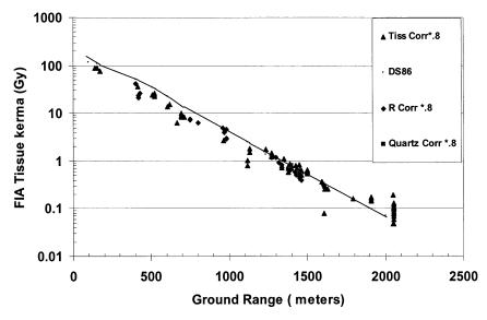
FIGURE 2-11 Hiroshima TL measurements (Corrected). Original reported units—roentgen, tissue, air, quartz—converted to FIA tissue kerma (Cullings 2000).
