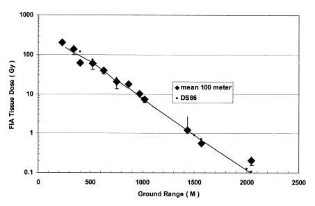
FIGURE 2-16 Nagasaki TL measurements averaged over 100-m intervals.
