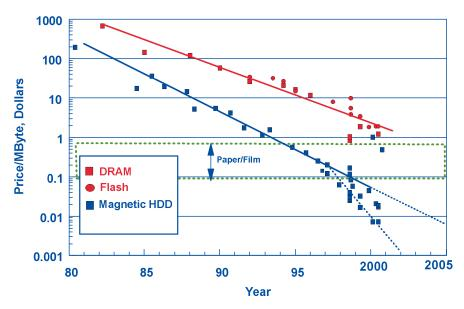
FIGURE 9.7 Cost per megabyte of magnetic hard disk drive (HDD) storage, 1980 to 2005 (projected). Semiconductor memory (Flash and DRAM) is shown for comparison. Courtesy of IBM Research.
