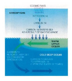
As cold, salty water sinks to great depths, as shown above, it carries radioactive <sup>14</sup>C out of the atmosphere and into the abyss, where it slowly decays. Radiocarbon dating is used to measure the state of the oceanic current system.
