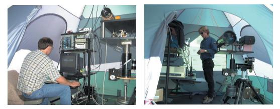
At the left is an operator sending a signal on the free-space transmitter; at the right, the signal, consisting of photons, is being received.
