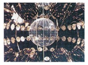
The BOREXINO neutrino detector (left) will for the first time allow us to see the elusive low-energy neutrinos from the decay of <sup>7</sup>Be in the Sun's core. This measurement will provide critical new data on the mass of the neutrino and its other properties.
