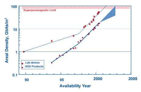
FIGURE 9.6 Hard disk drive (HDD) areal density is now doubling every 12 months. Courtesy of IBM Research.
