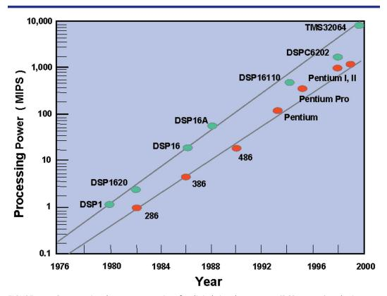
FIGURE 9.3 Computational power versus time for digital signal processors (DSPs, green) and microprocessors (red). Courtesy of Intel and Texas Instruments.
