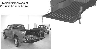
FIGURE 2-2 Polymer composite pickup box. SOURCE: Mehta, 2000.
