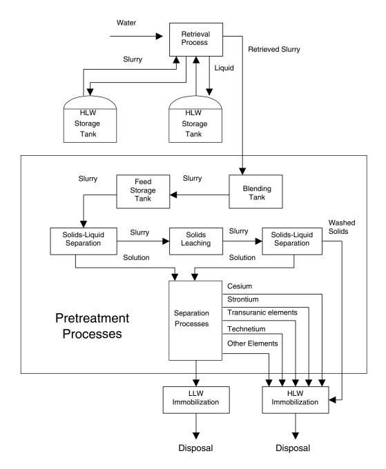
The first step consists of the retrieval of waste slurry from the tanks and the mixing of various batches of feed materials to achieve a reasonable volume of feed with uniform properties. SLS is performed to separate solids from the slurry, leaving a solids-free solution. This separation may recur at several points in the process. Sludge leaching consists of FIGURE 4.1 Simplified scheme of the pretreatment process.
