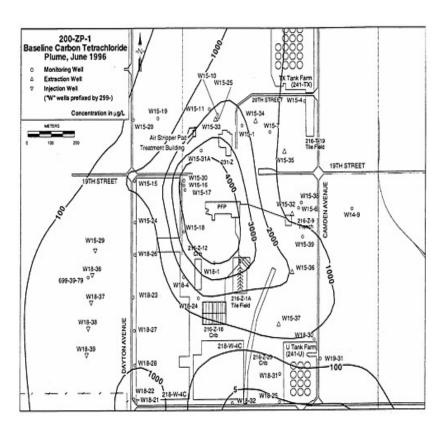
Figure 2.7 Map showing carbon tetrachloride groundwater plume concentration isopleths (in micrograms per liter) in the 200 West Area at the Hanford Site in June 1996. The building marked "PFP" is the Plutonium Finishing Plant. SOURCE: DOE, 2000e, Figure 3–8.
