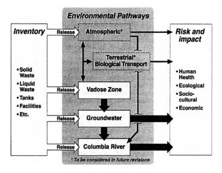
Figure 4.1 Conceptual illustration of the System Assessment Capability. SOURCE: Kincaid et al., 2000, Figure 1–1.
