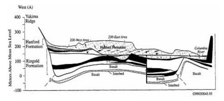
Figure 2.9 Generalized east-west section through the Hanford Site showing the principal geologic formations. SOURCE: PNNL, 1999, Figure 6.1.3.
