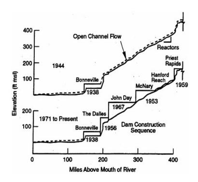
Figure 8.2 *Top:* Profile of the Columbia River channel bed in 1944. *Bottom:* Profile of the river channel at present. Dates on the figure indicate dam completion. NOTE: msl=mean sea level. SOURCE: BHI, 1999, Figure E-4.
