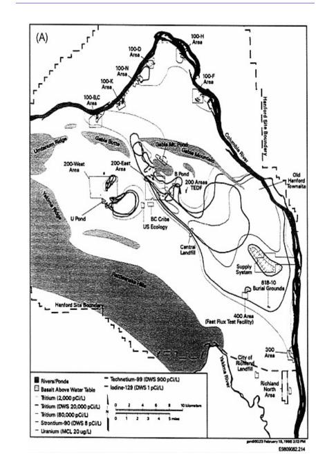
Figure 2.8 Boundaries of major groundwater plumes at the Hanford Site: (A) radionuclide plumes, (B) chemical plumes. SOURCE: DOE, 1998a, Figures 1-3 and 1-4.
