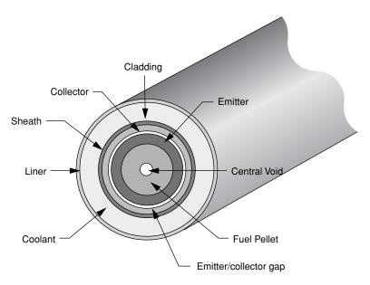
FIGURE 3.2 A cross sectional view of a thermionic fuel element (TFE). The nuclear fuel is located in the middle of the TFE and radiates heat outward.
