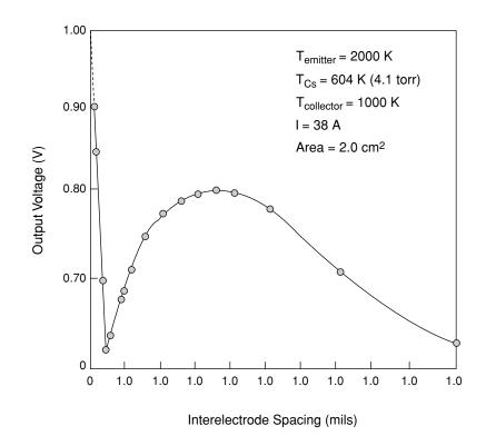
FIGURE 3.3 Solar thermionic output voltage based on emitter-collector spacing. SOURCE: Jet Propulsion Laboratory, Solar Energy Technology program unpublished data, circa 1967.
