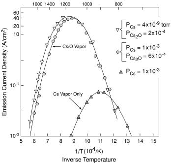
FIGURE 7.3 Effects of cesium oxide vapor on converter performance.
