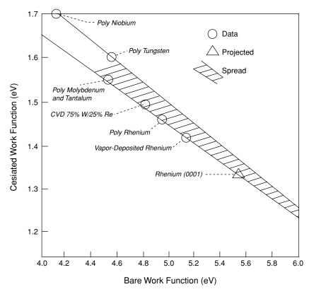
FIGURE 7.2 Cesiated work function versus bare work function.
