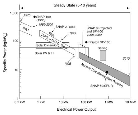
FIGURE 3.6 Inverse specific mass versus electrical power output.
