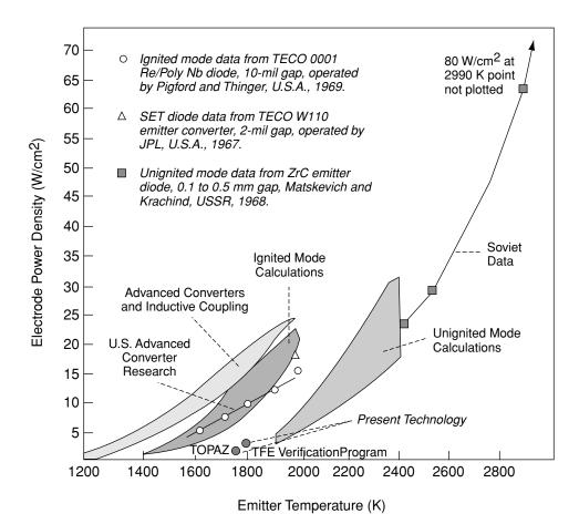
FIGURE 3.7 Increase in power density of a nuclear thermionic system as a function of temperature.
