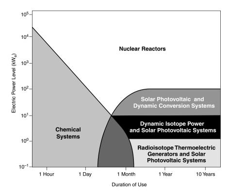
FIGURE 3.5 Power system options for specific mission durations.
