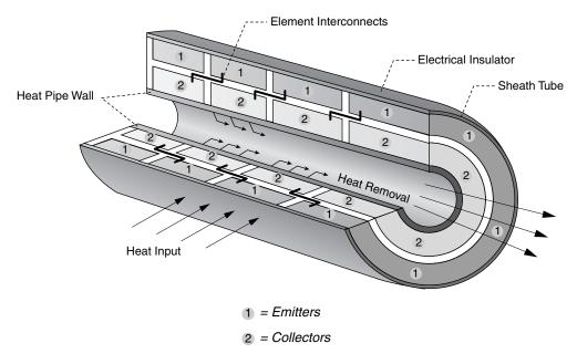
FIGURE 5.1 Cylindrical inverted multicell cross section. SOURCE: L. Begg, General Atomics, presentation to the Committee on Thermionic Research and Technology, August 2000.
