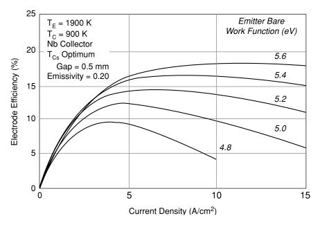
FIGURE 7.1 Effect of emitter bare work function on performance, using computer code TECMDL. SOURCE: General Atomics.
