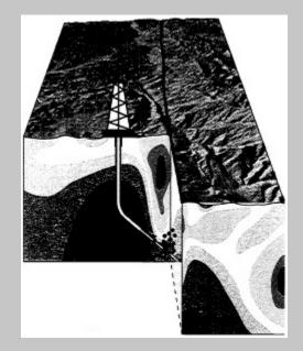
**Figure 2.** Schematic showing the planned SAFOD drillhole through the San Andreas fault zone near Parkfield, CA. In addition to providing rock and fluid samples, geophysical instrumentation emplaced deep in the drillhole will improve understanding of the nature of fault movement and earthquake activity by creating a long-term fault observatory (from EarthScope Working Group, 2001; EarthScope—A New View into Earth).
