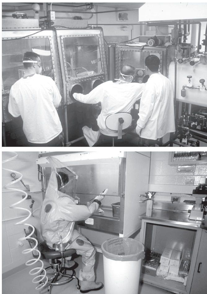
FIGURE 6.1 Different work modes in a BSL-4 laboratory at USAMRIID. At the top, hazardous samples are enclosed in a Class III Biological Safety cabinet. Below, the samples are more exposed in a Class II cabinet, but the worker is protected from them by a spacesuit. Using a glove box (Class III cabinet) is preferable for repetitive tasks that require limited lateral mobility. The spacesuit offers more flexibility, but at the cost of increased fatigue. SOURCE: Photographs courtesy of Steve Ferendo, USAMRIID.
