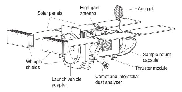
FIGURE 1. Schematic of the Stardust spacecraft with sample return capsule and other key parts marked.
