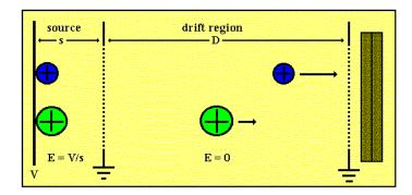
FIGURE 1. Diagram of a TOF mass spectrometer.
