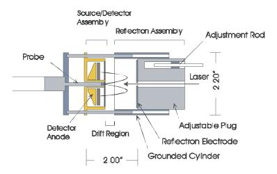
FIGURE 2. Diagram of endcap reflectron TOF mass spectrometer.
