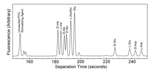
FIGURE 2. Baseline resolution of several amino acid enantiomers using the μCE chip system. SOURCE: L.D. Hutt, D.P. Glavin, J.L. Bada, and R.A. Mathies, "Microfabricated Capillary Electrophoresis Amino Acid Chirality Analyzer for Extraterrestrial Exploration," *Anal. Chem.* 71:4000-4006, 1999.
