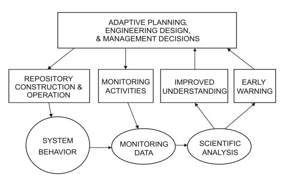
FIGURE 4.4 Role of monitoring during the operational phase of the repository. This figure indicates how monitoring interacts with management, construction, and operation activities and with the long-term science and technology program. Repository operations affect the system's behavior; changes in behavior, in turn, are detected by monitoring.
