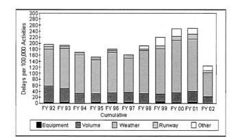
FIGURE 1–1. Cumulative causes of flight delays per 100,000 activities from 1992 to 2002.
