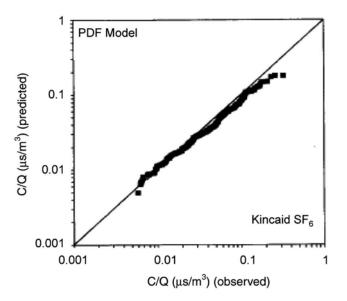
FIGURE 4.4 A Q-Q plot of the data in Figure 4.3. SOURCE: From Weil et al. (1997). Reprinted with permission from the American Meteorological Society.
