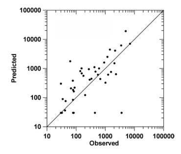
FIGURE 4.5 A dosage scatter plot for three-hour releases of sulfur hexaflouride (SF<sub>6</sub>). SOURCE: From Chang et al. (2003). Reprinted with permission from the American Meteorological Society.
