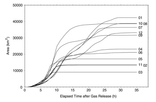
FIGURE E.2 Time evolution of the area with dosage above the threshold corresponding to the lowest value plotted in Plate 6. Area computations are limited to the part of the grid within the circle that is tangent to the sides of grid 3N, with a radius of 210 km (see arc in upper-left panel of Plate 6).
