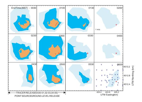
PLATE 8 Half-hour-average ground-level SF6 plume concentration measurements from intensive operation period (IOP) 10 of the URBAN 2000 field campaign in Salt Lake City, UT. Data are taken during the early morning of October 26, 2000.
