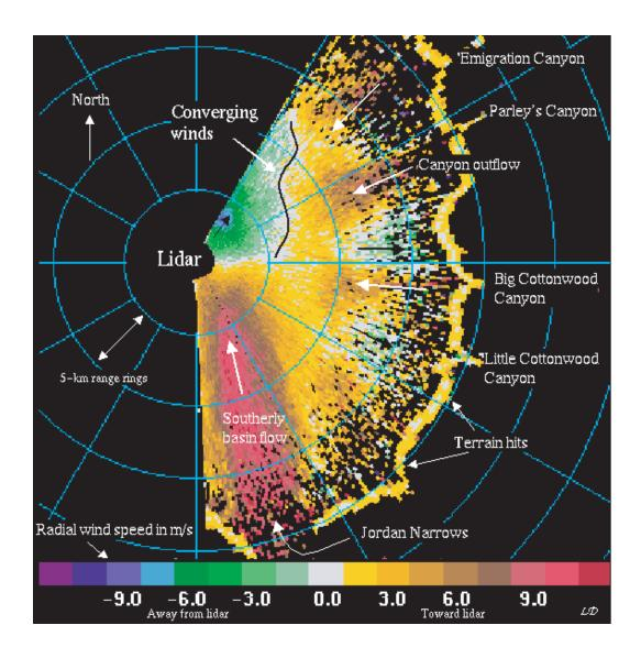
PLATE 5 Horizontal lidar scan that shows the complex air flow observed in the terrain around and south of Salt Lake City. SOURCE: Lisa Darby, NOAA/ETL.
