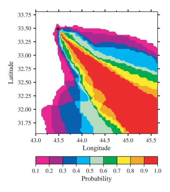
PLATE 7 Probability of the dosage exceeding 10-11 kg s m-3. The star symbol shows the location of the release.
