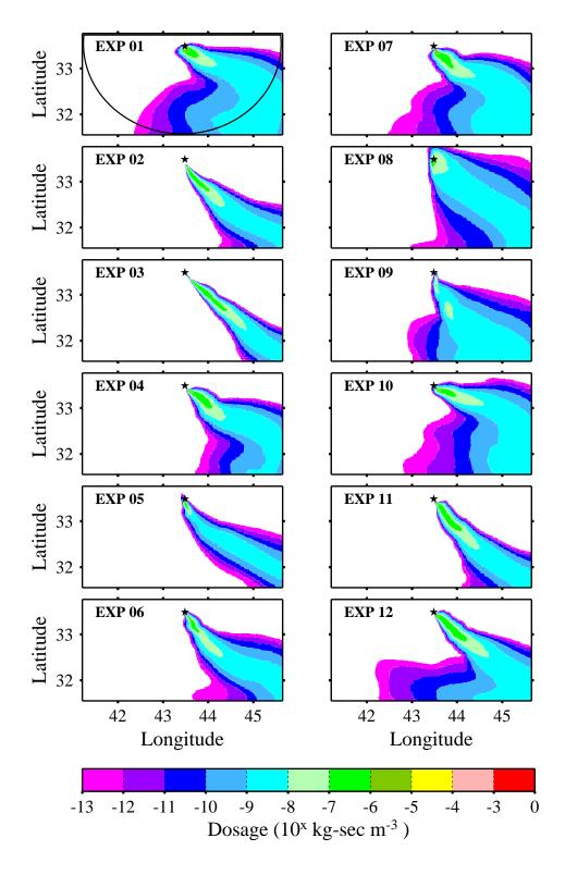
PLATE 6 Surface dosage after the released gas has exited the grid. The experiment numbers are listed in Table E.1. Note that the arc in the upper-left panel corresponds to a segment of the circle over which the area-above-dosage threshold values were calculated, which are displayed in Figure E.2.
