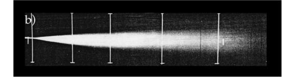
FIGURE 4.1 (a) A snapshot of the instantaneous plume downwind of a continuous source in a turbulent flow (horizontal cross section). (b) The time-averaged plume. (SOURCE: EPA Fluid Modeling Facility).
