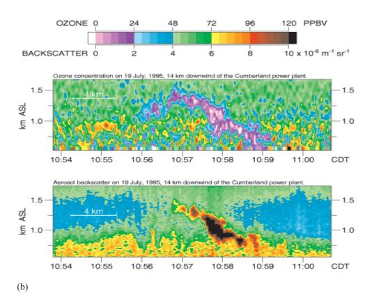
PLATE 1 Simultaneous images of a smoke plume via (a) camera and (b) remote sensing with lidar. SOURCE: (a) Shane Mayor, NCAR; (b) From Mayor et al. (1996). Reprinted with permission from Shane Mayor.
