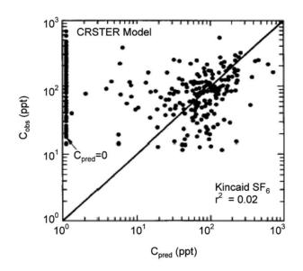
FIGURE 4.2 Observed versus predicted ground-level sulfur hexaflouride (SF<sub>6</sub>) concentrations for the CRSTER Gaussian plume model at the Kincaid power plant. The observations are one-hour averages. The diagonal line corresponds to  $C_{obs} = C_{pred}$ . SOURCE: From Weil et al. (1997). Reprinted with permission from the American Meteorological Society.
