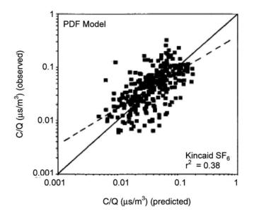
FIGURE 4.3 Observed versus predicted ground-level sulfur hexaflouride (SF<sub>6</sub>) concentrations, normalized with the emission rate, for the PDF model at the Kincaid power plant. PDF is an ensemble-average model with improved physics. The observations are one-hour averages. SOURCE: From Weil et al. (1997). Reprinted with permission from the American Meteorological Society.
