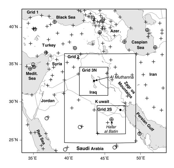
FIGURE E.1 Geographic extent of the computational grids. Grid 1 has a grid increment of 30 km, grid 2 has a grid increment of 10 km, and grids 3N and 3S have a grid increment of 3.3 km. The locations of surface (plus signs) and upper-air (circles) observations are also shown.
