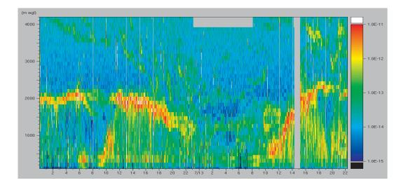
PLATE 3 Refractive index structure parameter ( $C_n^2$ ) inferred from the signal-to-noise ratio of the vertical beam of a 915-MHz radar profiler operating with a 700-ns pulse in East Brunswick, N.J., from 0 UTC 12 July 1997 to approximately 22 UTC 13 July 1997. The X-axis is time (hours), and the Y-axis is height above ground level (meters). The color bar shows the values of  $C_n^2$  (m<sup>-2</sup>). SOURCE: Tim Dye, Sonoma Technology Inc.
