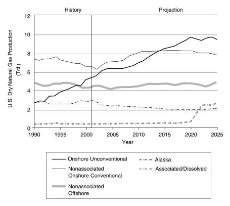
FIGURE 4.4 U.S. dry natural gas production in trillion cubic feet for the period 1990 to 2025. SOURCE: EIA (2003a, p. 76).
