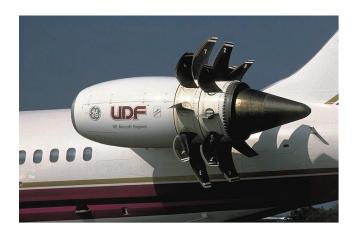
FIGURE 4-2 Unducted fan demonstrator ready for flight. Source: Burkhard Domke, Grünendeich, Germany. Available online at <www.b-domke.de/AviationImages/Rarebird/0809.html>.
