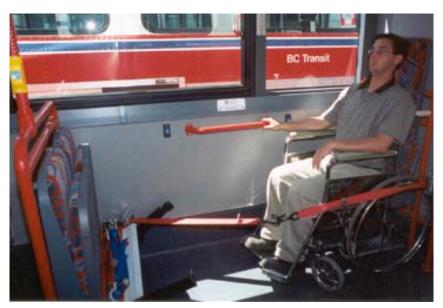
FIGURE 15 Combi 1 design on BC Transit double-decker bus with front- and rearfacing design in same position, and hooked straps to prevent tipping.
