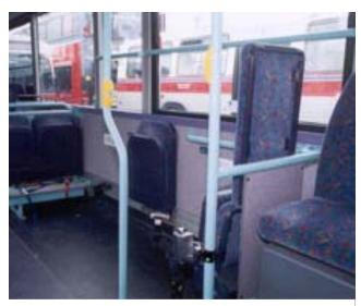
FIGURE 14 Combi system of forward and rear facing in one location, 10.6-m (35-ft) BC Transit low-floor bus (future standard for all buses).
