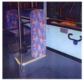
FIGURE 3 Rear-facing position with movable armrest (shown in up position). Instead of stanchion, there is a handrail on the wall and a separate stop request button (located below the handrail).
