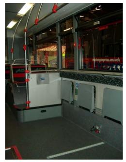
FIGURE 20 Forward-facing position (combi design) on prototype AC Transit BRT service bus.
