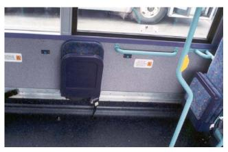
FIGURE 6 BC Transit rear-facing position with flip-down seats on bus wall and back panel.
