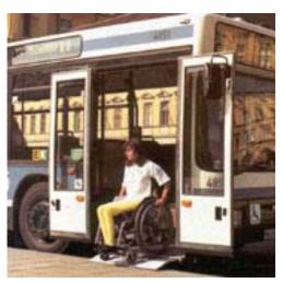
FIGURE 9 Access over ramp at front door (Germany).
