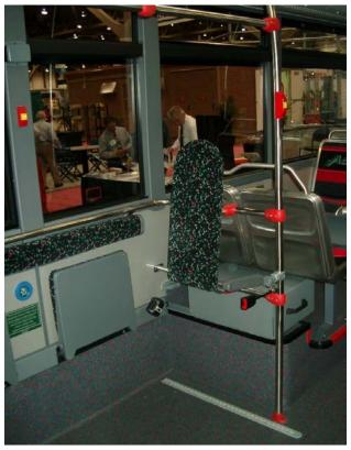
FIGURE 21 Rear-facing position (combi design) on prototype AC Transit BRT service bus.
