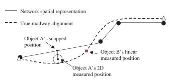
*Figure 3-8. Transformation of 2D-measured position to LR position.*
