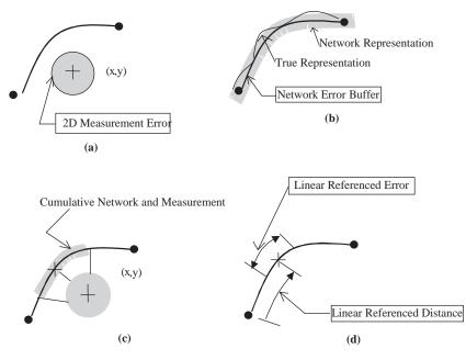
Figure 2-6. Schematic representation of positional data error.
