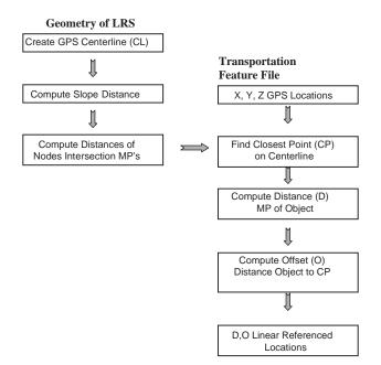
Figure 2-10. Steps in transformation of data for GPS to LRS.
