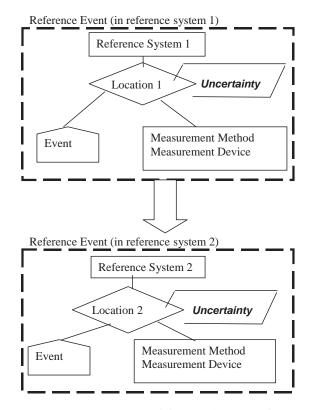
*Figure 2-13.* Data error model—transformation between referencing systems.
