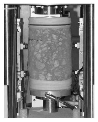
*Figure 7. Interlaken dynamic modulus test instrumentation.*
