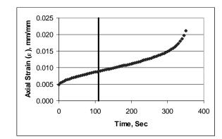
a. Axial Strain in Flow Time Test.
