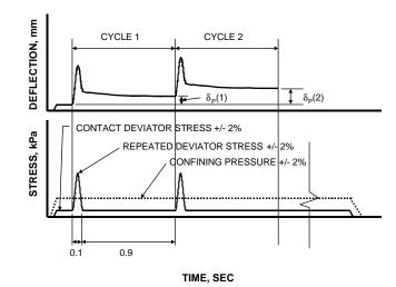
Figure 5. Schematic of Loading and Data Acquisition for Flow Time Test.
