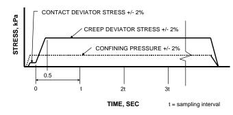
Figure 4. Schematic of Loading and Data Acquisition.
