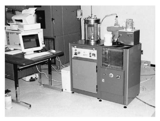
Figure 8. Shedworks simple performance test system.
