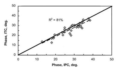
Figure 15. Comparison of phase angle values generated by the Interlaken (ITC) and Shedworks (IPC) simple performance test devices (dashed line represents fit, solid line equality).
