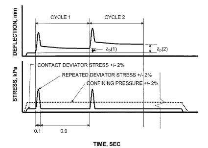
Figure 2. Schematic of flow number test loading.
