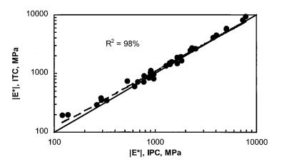
Figure 13. Comparison of dynamic modulus values generated using the Interlaken (ITC) and Shedworks (IPC) simple performance test devices (dashed line represents fit, solid line equality).
