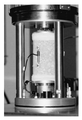
Figure 9. Shedworks dynamic modulus test instrumentation.
