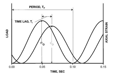
Figure 4. Typical dynamic modulus test data.
