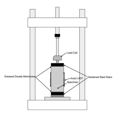
Figure 1. Schematic of Dynamic Modulus Test Device.
