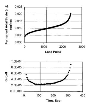
*Figure 3. Typical repeated load test response and flow number.*
