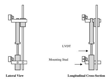
Figure 3. Mounting Hardware Details.
