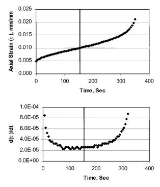
Figure 1. Typical creep test response and flow time.
