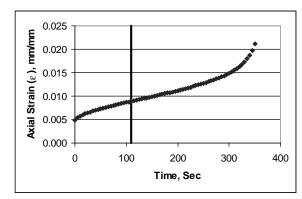
a. Axial Strain in Flow Time Test.
