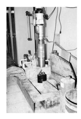
Figure 3. Portable Core Drilling Machine and Stand.
