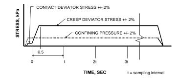
Figure 5. Schematic of Loading and Data Acquisition.
