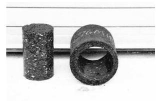
Figure 4. 100 mm Diameter Core and Waste Ring.
