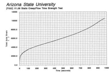
Figure 3. Total Axial Strain Vs. Time From a Static Creep / Flow Time Test.
