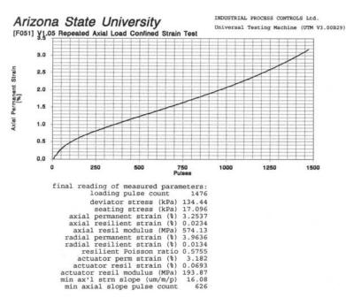
Figure 3. Cumulative Permanent Strain Vs. Loading Cycles From a Repeated Load
