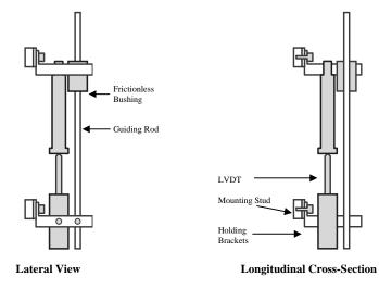
Figure 2. Axial LVDTs Instrumentation.
