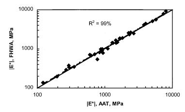
Figure 14. Comparison of complex modulus values generated at FHWA and at AAT using the two simple performance test devices (dashed line represents fit, solid line equality).
