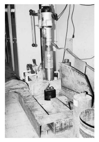
Figure 11. Portable core drilling machine and stand.
