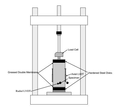
Figure 1. Schematic of Static Creep / Flow Time Test.
