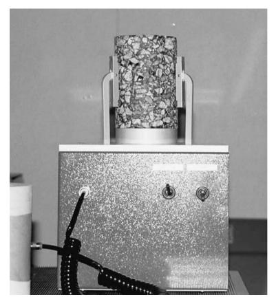
Figure 10. Shedworks glue-on gauge point system.
