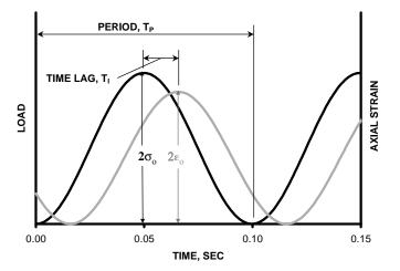
Figure 3. Schematic of Dynamic Modulus Test Data.
