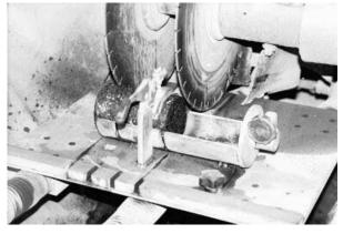
Figure 5. Double Bladed Saw With 100 mm Core.
