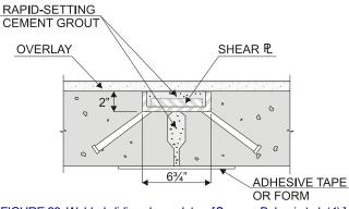
FIGURE 23 Welded sliding shear plates. [Source: Babaei et al. (1).]
