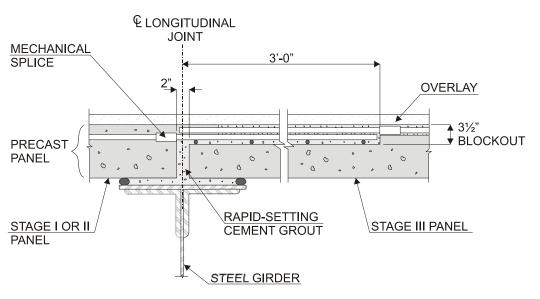
FIGURE 24 Longitudinal connections. [Source: Babaei et al. (1).]
