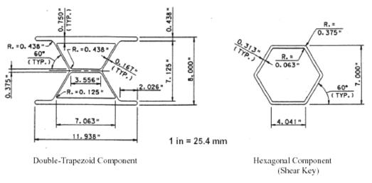
FIGURE 47 Cross section of composite bridge deck. [Source: Shekar et al. (34).]
