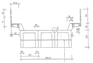
FIGURE 9 Channel-type girder railway bridge.
