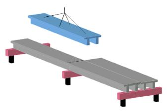
FIGURE 32 Double-tee bridge system.
