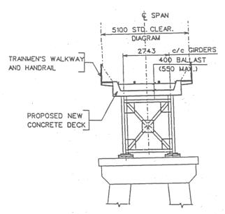
FIGURE 6 Steel deck plate girder railway bridge with prefabricated prestressed concrete slab.
