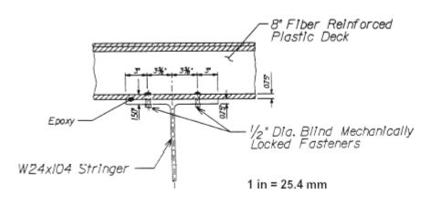
FIGURE 49 Deck to stringer connection using BOM blind bolts. [Source: Shekar et al. (34).]
