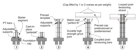
FIGURE 39 Erection sequence for a single-column bent. [Source: Billington et al. (21).]
