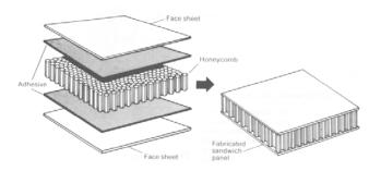
FIGURE 45 Sandwich construction.
