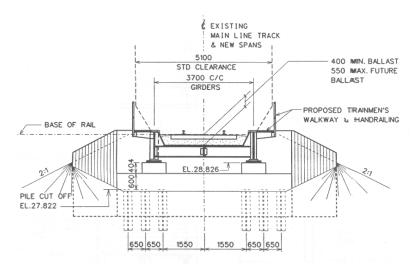
FIGURE 7 Through plate girder railway bridge deck.
