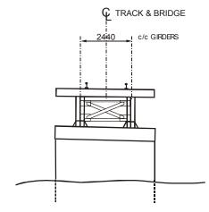
FIGURE 5 Open deck steel span railway bridge.
