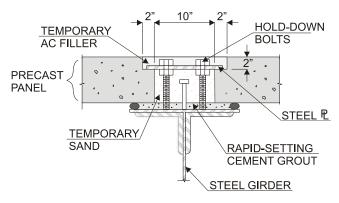
FIGURE 27 Temporary panel restraint for traffic. [*Source*: Babaei et al. (1).]
