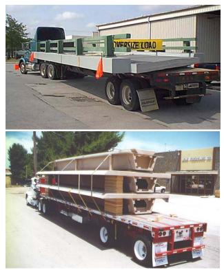
FIGURE 2 Fabrication and transportation of FRP bridge segments.
