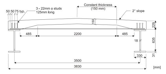
FIGURE 12 Typical cross section of experimental arch panel on steel support beams.
