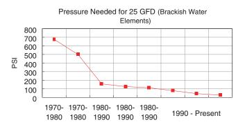
FIGURE 10.5 Historical reduction in operating pressure for Dow's reverse osmosis membranes.
