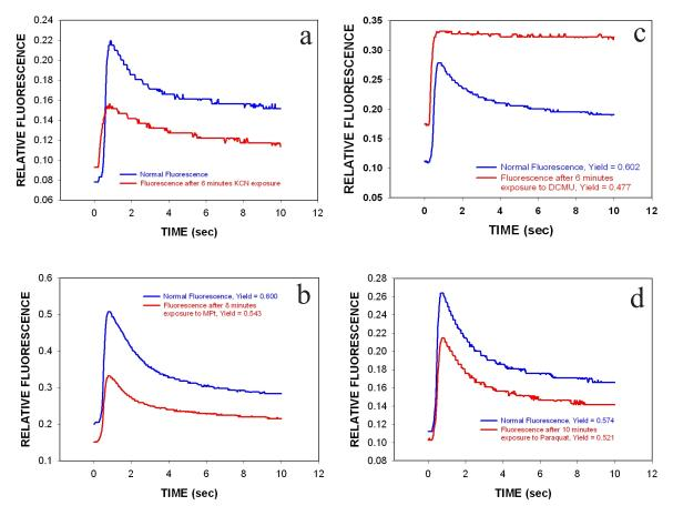
FIGURE 6.2a-d Effect of 2 mM KCN, 20 µM MPt, 10 µM DCMU, and 30 µM Paraquat, respectively, on time-resolved fluorescence signal of naturally occurring algae from the Clinch River. There is a six-minute delay between collection of the two curves in each plot shown. In plots a-c, the top curve shows is the normal fluorescence trace of the water sample, while for plot d it is the bottom curve. Time zero is the initiation of fluorescence excitation of the sample measured.
