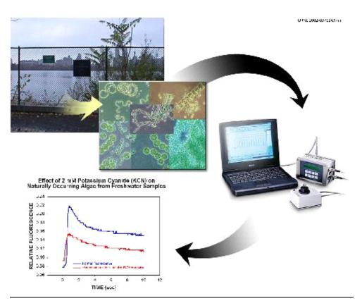
FIGURE 6.1 AquaSentinel: a continuous water monitoring system using naturally occurring algae as biosensors.
