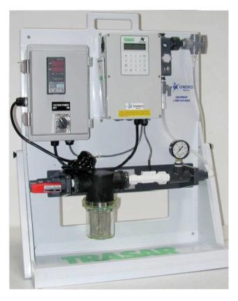
FIGURE 9.12 TRASAR for RO scale control.
