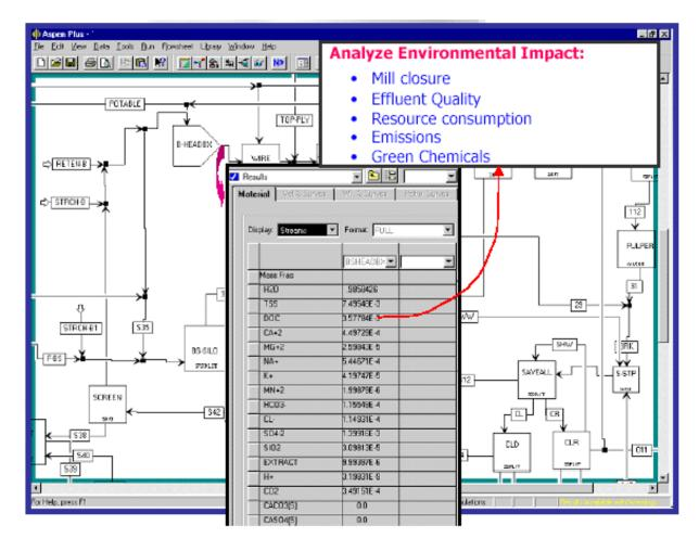
FIGURE 9.10 Virtual paper machine model.
