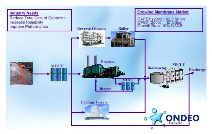
FIGURE 9.13 Twenty-first century industrial water management and the role of membrane separations technology.
