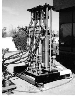
FIGURE 4.8 The VARI-RO positive displacement process and pilot plant.
