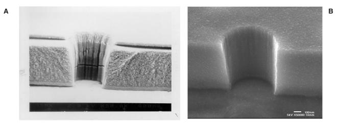
FIGURE 2.1 Comparison of a semiconductor component showing sidewall polymer (A) prior to cleaning, and (B) after cleaning with supercritical  $CO_{2}$ .
