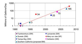
FIGURE 10.7 Reverse osmosis membrane facilities—largest plants as a function of time, with nanofiltration (NF), seawater (SW), and brackish water (BW).
