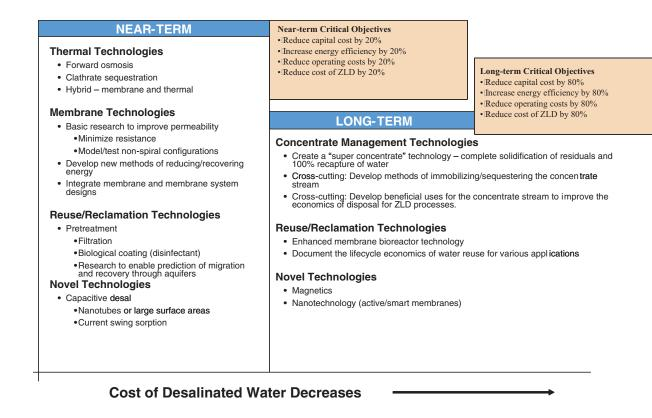
FIGURE 4.7 Technologies related to desalination objectives
