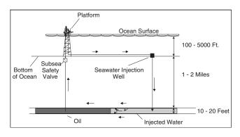
FIGURE 10.8 Nanofiltration membranes remove sulfate ions that could precipitate from water injected into oil reservoirs from off-shore platforms.
