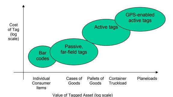
**FIGURE 1.1** The types of tags appropriate for different types of assets. Both the vertical scale of tag cost and the horizontal scale of asset value are logarithmic.
