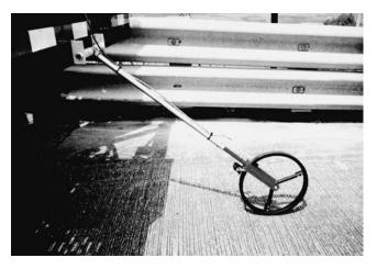
*Figure 26. Surveyors wheel mounted to rear bumper of truck.*
