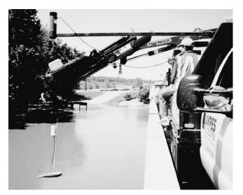
Figure A23. Wireless sonar in a sounding weight.
