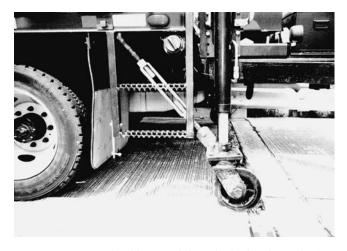
*Figure 34. Turnbuckle to stabilize the hydraulic jacks for the crane.*
