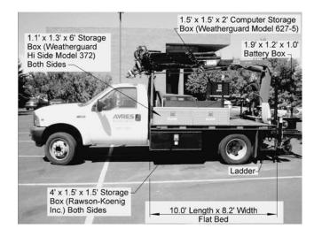
Figure A8. Truck bed and toolbox dimensions.
