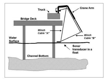
*Figure 7. Two winch concept for cable suspended operations.*
