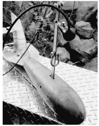
Figure B7. Marsh-McBirney velocity sensor on a 50 lb sounding weight.
