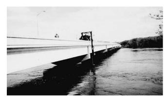
Figure 48. Arc measurements on the upstream side of Wisconsin STH80, pier 1.
