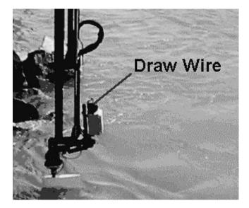
Figure A12. Draw wire to measure the extension of the crane.
