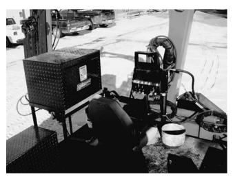
*Figure 21. Instrument shelter for computer and relocated hydraulic controls.*
