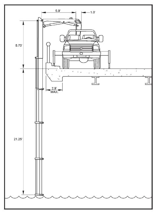
Figure A3. Reach below the bridge deck with the PK4501C crane on a Ford F-450 truck.
