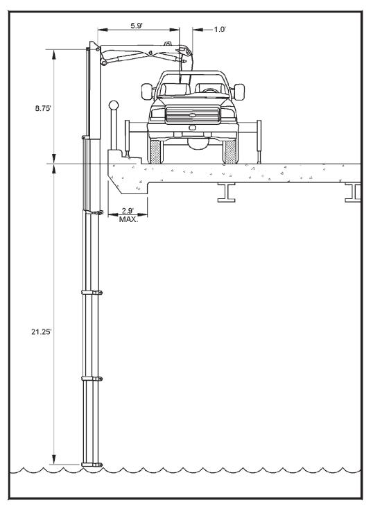
Figure 17. Reach below the bridge deck with the PK4501C crane on a Ford F-450 truck.
