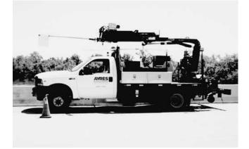
*Figure A4. PK4501C crane mounted on the back of a F450 truck.*
