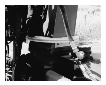
*Figure 22. Attachment for crane azimuth measurement using draw wire.*
