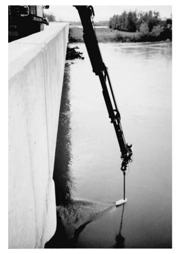
Figure 51. Arc measurement at pier 5, U.S. 24.
