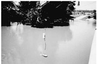
Figure B33. Sounding weight with sonar.
