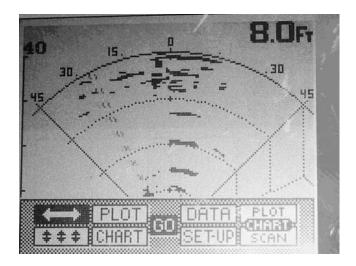
Figure 13. Horizontal scan showing multiple reflections.
