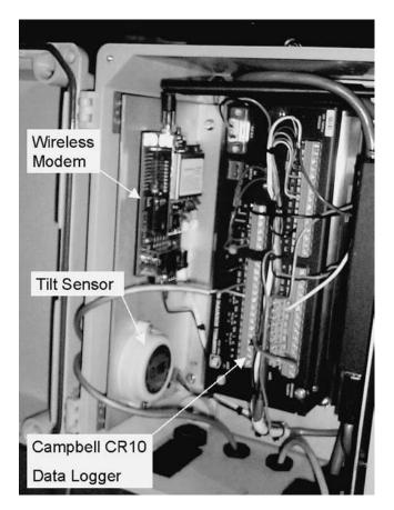
*Figure 23. Tiltmeter installed in the instrument box at the end of the crane.*
