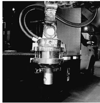
*Figure A6. Standard rotator (prior to modifications to allow tilt).*
