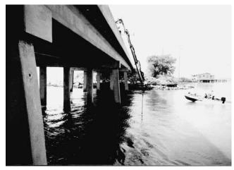
*Figure B10. Making an arc measurement on the Gulf side of the bridge.*
