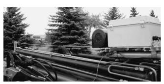
*Figure 24. Draw wire used to measure linear extension of crane.*
