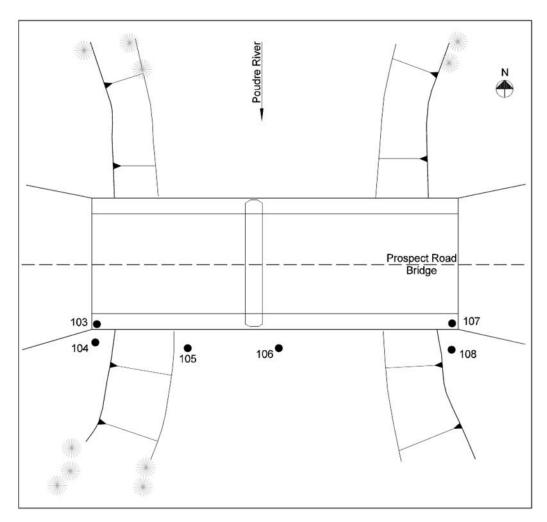
Figure 36. Control grid for GPS testing.
