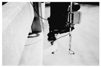
*Figure B13. Marsh-McBirney current meter mounted on the crane upstream of the sonar.*
