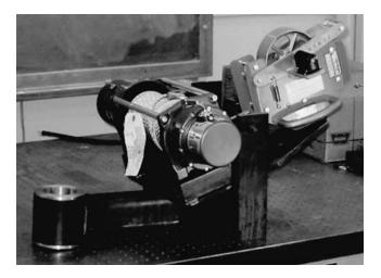
Figure 8. Modified winch design.
