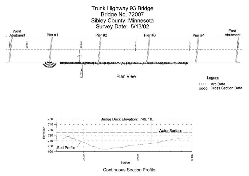
Figure B18a. Minnesota Trunk Highway 93 cross section results.
