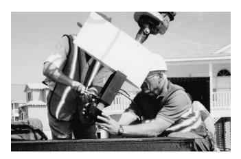
Figure 14. Mounting the Twinscope<sup>TM</sup> transducer for field testing.
