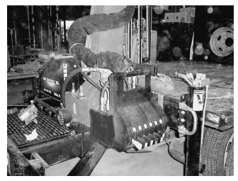
*Figure 20. Hydraulic controls in typical location allowing operation from roadway.*
