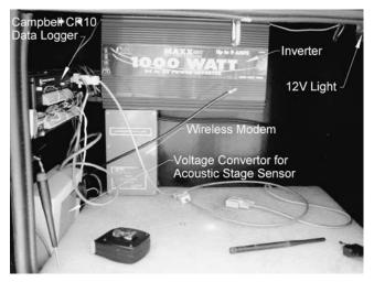
Figure A15. Inside view of instrument shelter on truck bed.
