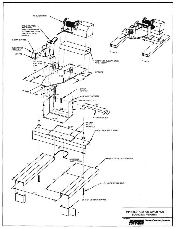
Figure 6. Dimensioned drawing of Minnesota style winch.
