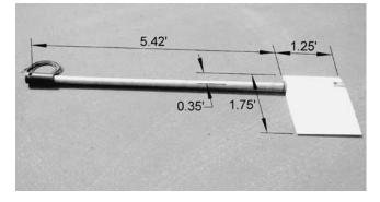
Figure A17. Streamlined sonar probe.
