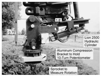
Figure A7. Rotator after modifications to provide tilt.
