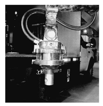
*Figure 18. Standard rotator (prior to modifications to allow tilt).*
