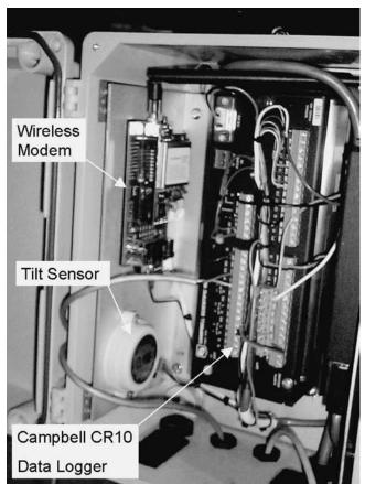
Figure A11. Instrument box at the end of the crane.
