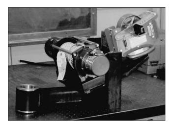
*Figure A21.* Winch and wire rope counter on mounting bracket.
