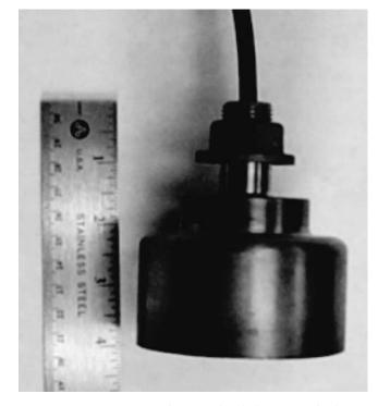
*Figure 27.* Sonar transducer with all electronics built into the transducer head.
