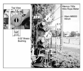
Figure A22. Post mounting design for dual winches.
