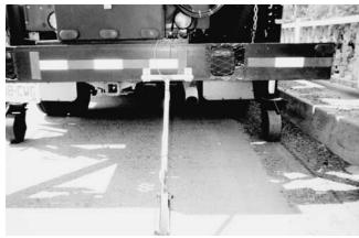
*Figure B40.* Castor movement through sand and gravel deposited along curbline.
