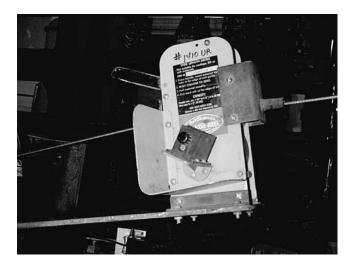
Figure 4. Close-up of Hykon— $ReeI^{TM}$  with guide added at the outlet of the reel.
