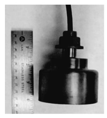
*Figure A16. Sonar transducer with all electronics built into the transducer head.*
