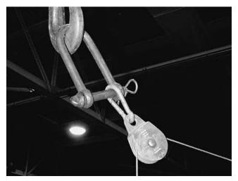
Figure 5. Pulley at end of articulated crane.
