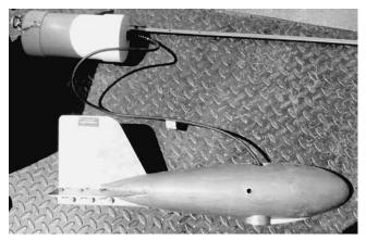
*Figure B34. Close up of sounding weight showing wedge on leading edge of sonar.*
