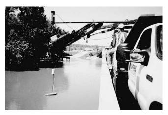
*Figure 53. Sounding weight with a wireless sonar being tested in Indiana.*
