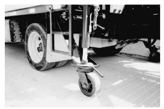
Figure 35. Final design for castor system.
