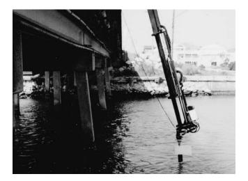
Figure 15. Positioning the Twinscope<sup>TM</sup> transducer upstream of a pile.
