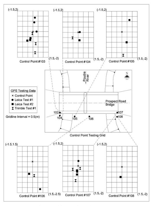
Figure 39. Error in the measured data at each control point.
