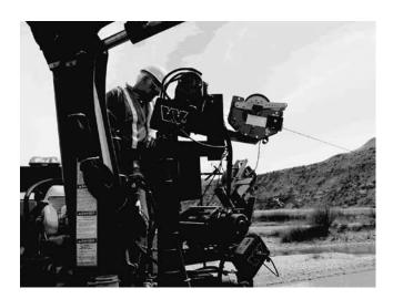
Figure B6. Using a single winch to position sounding weight with Marsh-McBirney.
