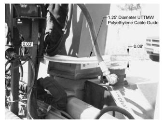
Figure A10. Draw wire attachment to base of crane.
