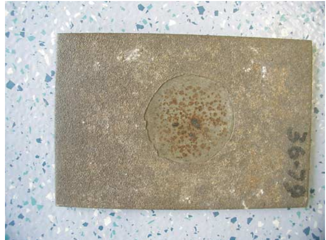
Figure 39. Cyclic (alternate) immersion panels with circular holidays after 6 months in test (zinc TSMC on left and aluminum TSMC on right).
