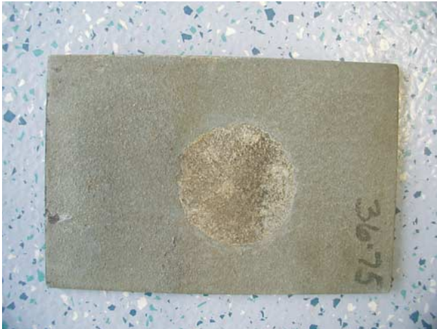
Figure 39. Cyclic (alternate) immersion panels with circular holidays after 6 months in test (zinc TSMC on left and aluminum TSMC on right).
