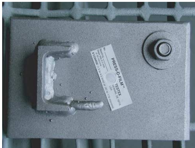
Figure 6. Testex tape to evaluate surface profile.
