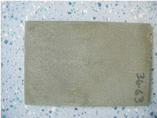
Figure 40. Cyclic (alternate) immersion panels with scribes after 6 months test (zinc TSMC on left and aluminum TSMC on right).
