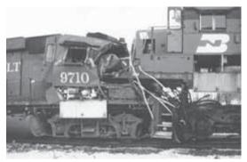
Scenario 1 locomotive crash near Smithfield, West Virginia, August 20, 1996—collision with a 28car train traveling at 24 mph caused the trailing locomotive of a 41-car train traveling at 22 mph to override the leading locomotive.
