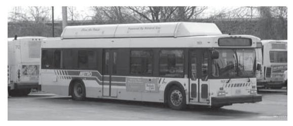
CNG-powered bus in Akron (Ohio) Metro system; the CNG fuel cylinders are mounted on the bus roof, beneath the housing.
