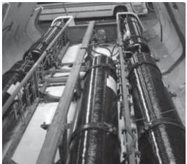
CNG fuel cylinders, fuel lines, and safety devices under bus roof.
