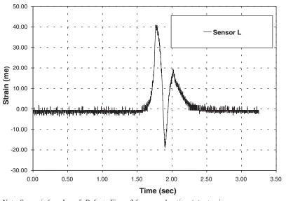
Note: Sensor is from Lane 5. Refer to Figure 2 for sensor location. (+) = tension.
