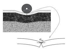
FIGURE B24 Joint spalling mechanism in ALF.
