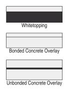
FIGURE 1 Concrete overlay types.
