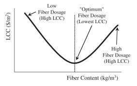
FIGURE 6 Optimizing fiber content using LCC.
