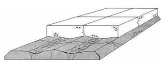
FIGURE 17 With an uneven HMA, err on the thick side (82).
