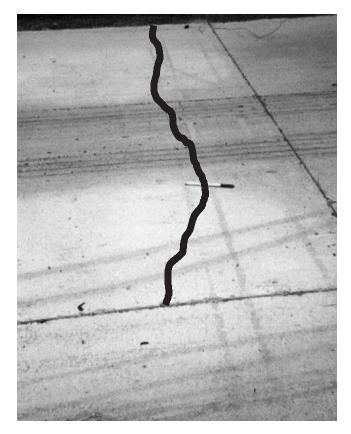
FIGURE B12 Typical UTW transverse cracking at the FHWA ALF.
