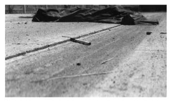
FIGURE B14 Typical UTW longitudinal faulting at the FHWA ALF.
